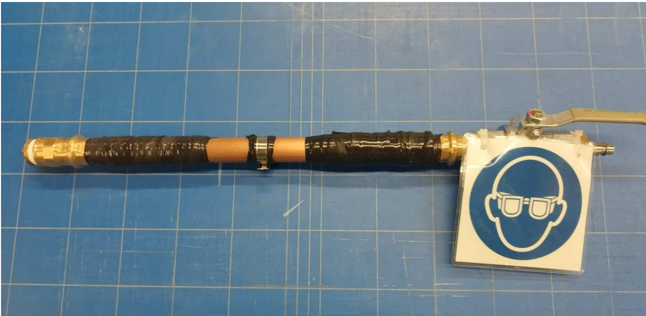
Figure 1: Test tube wrapped with tesa® 4600
