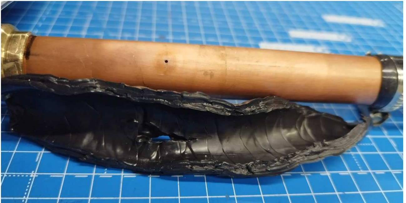
Figure 5: Failed sample #1 after removal from the tube
