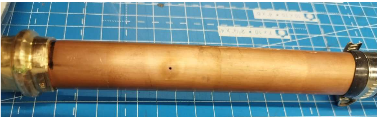
Figure 2: Tube with the hole (D=1mm) for leakage simulation
