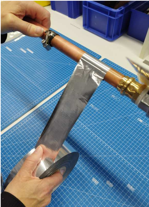
Figure 3: Application of Alu-tape tesa® 60634
