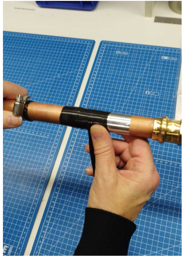
Figure 4: Application of tesa® 4600
