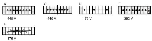
Max voltage data with optional screen bus bar LS 2.5
