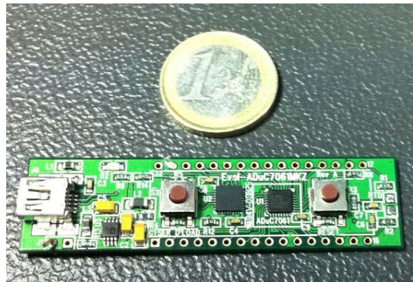
Figure 2. EVAL-ADuC7061MKZ Board Used for this Circuit.
