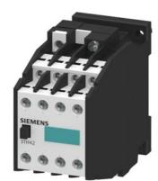
Contactor relay, 44E, DIN EN 50011, 4NO + 4NC, screw terminal AC operation 230 V AC 50/60 Hz
