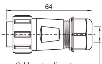
Cable outer diameter range: 7-12mm
