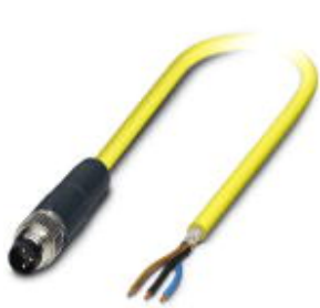
Sensor/Actuator cable, 3-position, PVC, yellow, shielded, Plug straight M8, on Free cable end, Cable length: 10 m
