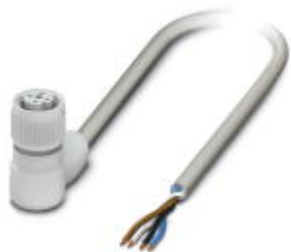
Sensor/Actuator cable, 4-position, PP-EPDM halogen-free, Gray RAL 7035, free cable end, on Socket angled M12, A-coded, Cable length: 3 m, Hygienic design, with plastic knurl
