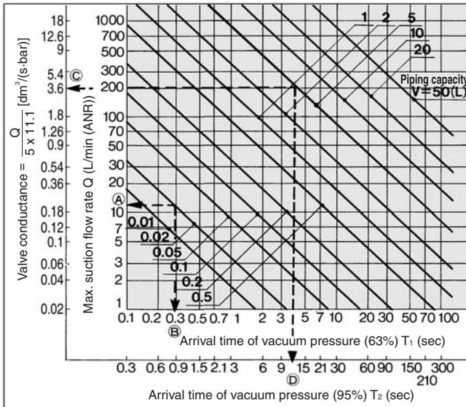
\* Conversely, the size of the ejector or the size of the switching valve of the vacuum pump system can be obtained from the adsorption response time.
