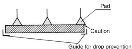
Provide an auxiliary device (example: a guide for preventing the workpieces from dropping) as necessary.
