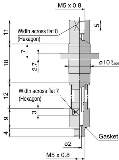
\* Refer to the front matter 30 for nut tightening torque.
