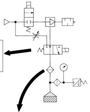
Use a suction filter (Series ZFA, ZFB, ZFC) to protect the switching valve and to prevent the ejector from becoming clogged. Also, a suction filter must be used in a dusty environment. If only the unit's filter is used, it will become clogged quickly.
