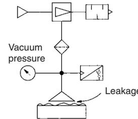
If a considerable amount of leakage occurs between the workpiece and the pad, resulting in incomplete adsorption, or to shorten the adsorption and transfer time, select an ejector nozzle with a larger diameter from the ZH, ZM, ZR, or ZL series.
