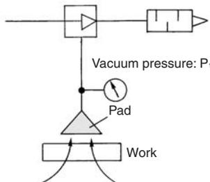
**Exercise:** Using a supply pressure of 0.45 MPa, when the ejector (ZH07□S) picks up a workpiece that leaks air, the vacuum gauge indicated a pressure of -53 kPa. Calculate the leakage volume from the workpiece.
