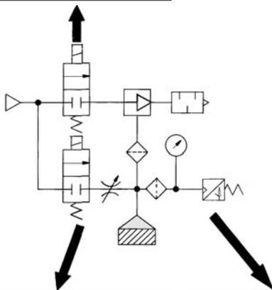
For the release valve, select a 2/3 port valve with a low vacuum specification. Also, use a needle valve to regulate the release flow rate.
