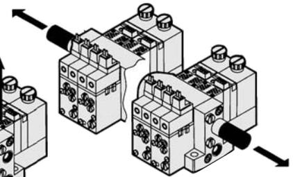
If there are a large number of ejectors that are linked on a manifold and operate simultaneously, use the built-in silencer type or the port exhaust type.
