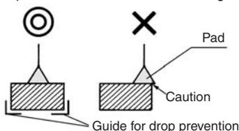
If multiple pads are used for transferring a flat object with a large surface area, properly allocate the pads to maintain balance. Also make sure that the pads are aligned properly to prevent them from becoming disengaged along the edges.
