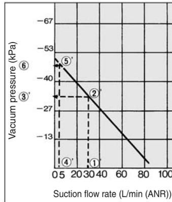
The vacuum pressure varies in accordance with the leakage volumes indicated in the above diagrams.
