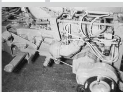
Picture 2.4: Vibrations, dirt, and temperatures up to 130°C occur in the area surrounding the engine
