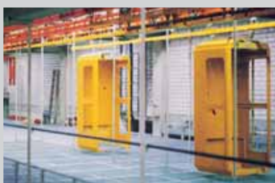
Picture 2.5: Conveyor chains: Through edge loading, short term surface pressures of over 50 MPa can occur
