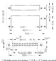
1) Solder pins for holes  $\varnothing$  0.8 + 0.3 mm on request
