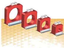
LTRC Series – Resin Cast CT's are Epoxy Resin type with Insulation Class E (120°C). These LV metering CT's feature sealable terminal covers and primary current ratings from 100A to 1200A. Available in various, Bus bar sizes, case widths, and with foot mounting facility.
