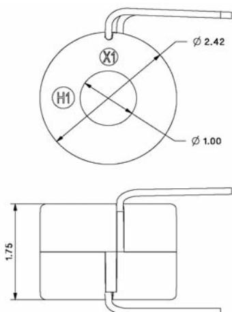
Used for ammeter, Wattmeters & cross current compensation
