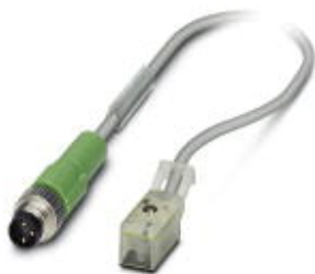
Sensor/actuator cable, 2-position, PUR, Gray RAL 7001, Plug straight M8, on Valve connector Festo KMYZ9, with 1 LED, Cable length: 5 m
