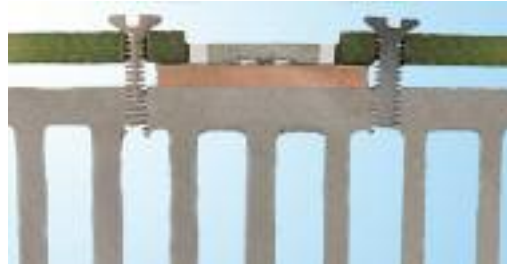
Sectional view shows sandwich of ACULED with TL-PCB mounted on standard heat sink
