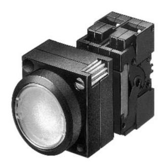
22MM PLASTIC ROUND COMPLETE UNIT COMBINATION: ILLUMINATED PUSHBUTTON MOMENTARY CONTACT TYPE WITH FLAT BUTTON ILLUMINATED WITH INTEGRATED LED 230V AC SCREW TERMINAL, 1NO+1NC WITH HOLDER GREEN
