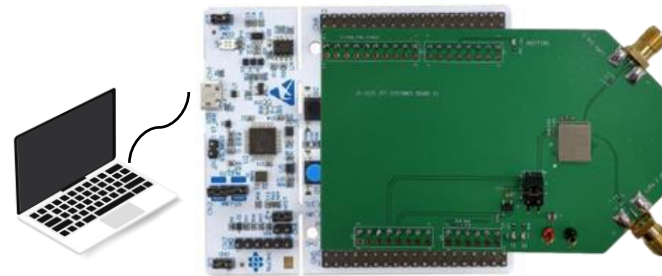
Figure2: connection to the PC
