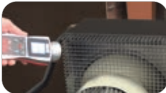
Stroboscope off: rotations not visible
