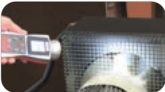
Stroboscope on: rotations visible
