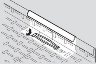
4. The second leg is pushed towards the wall of the tray and pushed home into the same slot
