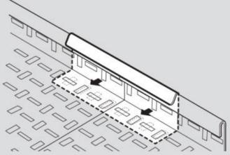
1. Locate coupler across underside of tray joint
