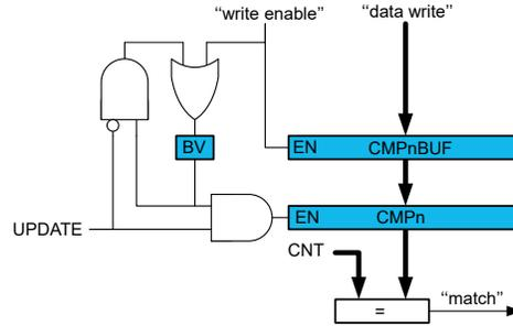
Both the TCA<sub>n</sub>.CMP<sub>n</sub> and TCA<sub>n</sub>.CMP<sub>n</sub>BUF registers are available as I/O registers, allowing the initialization and bypassing of the buffer register and the double-buffering function.
