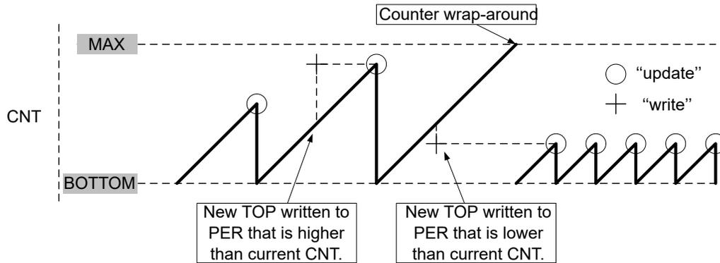
A counter wrap-around can occur in any mode of operation when counting up without buffering, as the TCA<sub>n</sub>.CNT and TCA<sub>n</sub>.PER registers are continuously compared. If writing a new TOP value to TCA<sub>n</sub>.PER lower than the current TCA<sub>n</sub>.CNT, the counter will wrap first before a compare match occurs.
