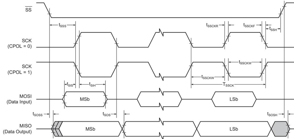
Table 35-20. SPI - Timing Specifications in Client Mode
