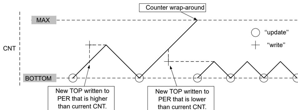
**With Buffering:** When using double-buffering, the buffer can be written at any time and still maintain the correct operation. TCA<sub>n</sub>.PER is always updated on the UPDATE condition, as shown
