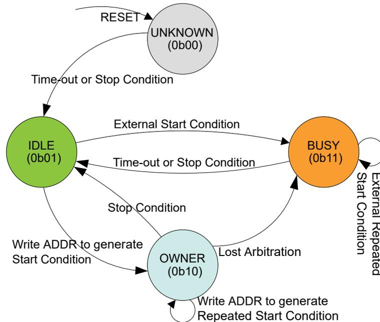
1. **Unknown:** The bus state machine is active when the TWI host is enabled. After enabling the TWI host, performing a system Reset, or disabling the TWI host, the bus state is Unknown.
