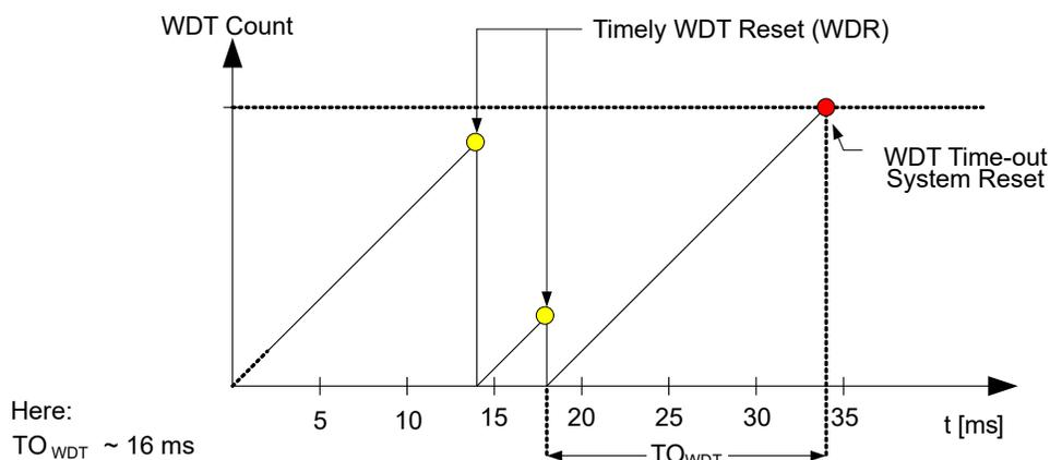
The Normal mode is enabled as long as the Window (WINDOW) bit field in the WDT.CTRLA register is '0x0'.
