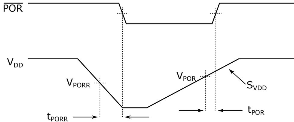
**Note:** When  $\overline{\text{POR}}$  is low, the device is held in Reset.
