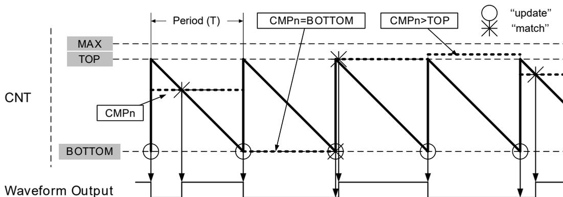
**Note:** The maximum duty-cycle of the waveform output is  $TOP/(TOP+1)$ .
