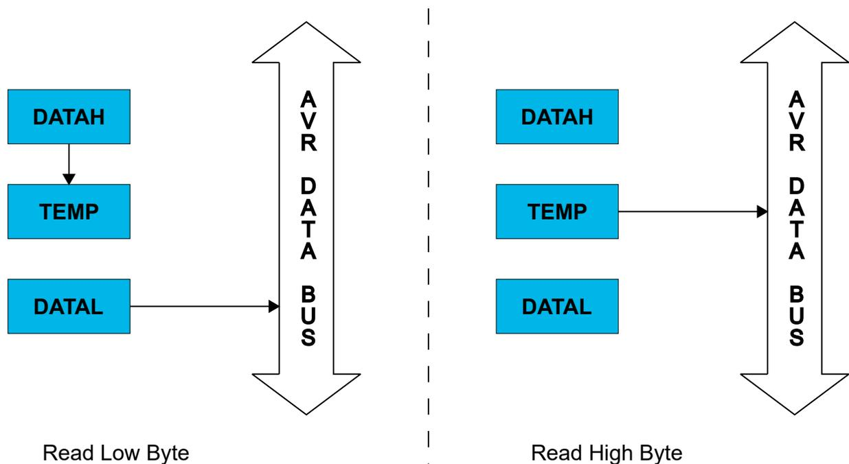
For a 16-bit read operation, the low byte register (e.g., DATAL) of the 16-bit register must be read before the high byte register (e.g., DATAH). When the low byte register is read, the high byte register of the 16-bit register is copied into the temporary (TEMP) register in the same clock cycle, as shown on the left side of the figure above. Reading the high byte register will result in a read from TEMP instead of the high byte register, as shown on the right side of the same figure.
