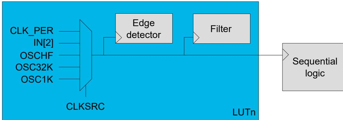
When the Clock Source (CLKSRC) bit is written to  $0 \times 1$ , LUTn-TRUTHSEL[2] is used to clock the corresponding filter and edge detector (CLK\_LUTn). The sequencer is clocked by the CLK\_LUTn of the even LUT in the pair. When CLKSRC is written to  $0 \times 1$ , LUTn-TRUTHSEL[2] is treated as OFF (low) in the TRUTH table.
