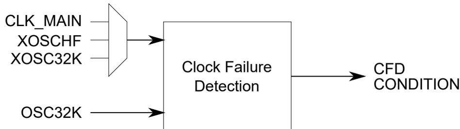
When the CFD feature is enabled, it will monitor the selected source from the Clock Failure Detection Source (CFDSRC) bit field in the Main Clock Control C (CLKCTRL.MCLKCTRLC) register. In sleep, the CFD will only be enabled if the selected source is active.
