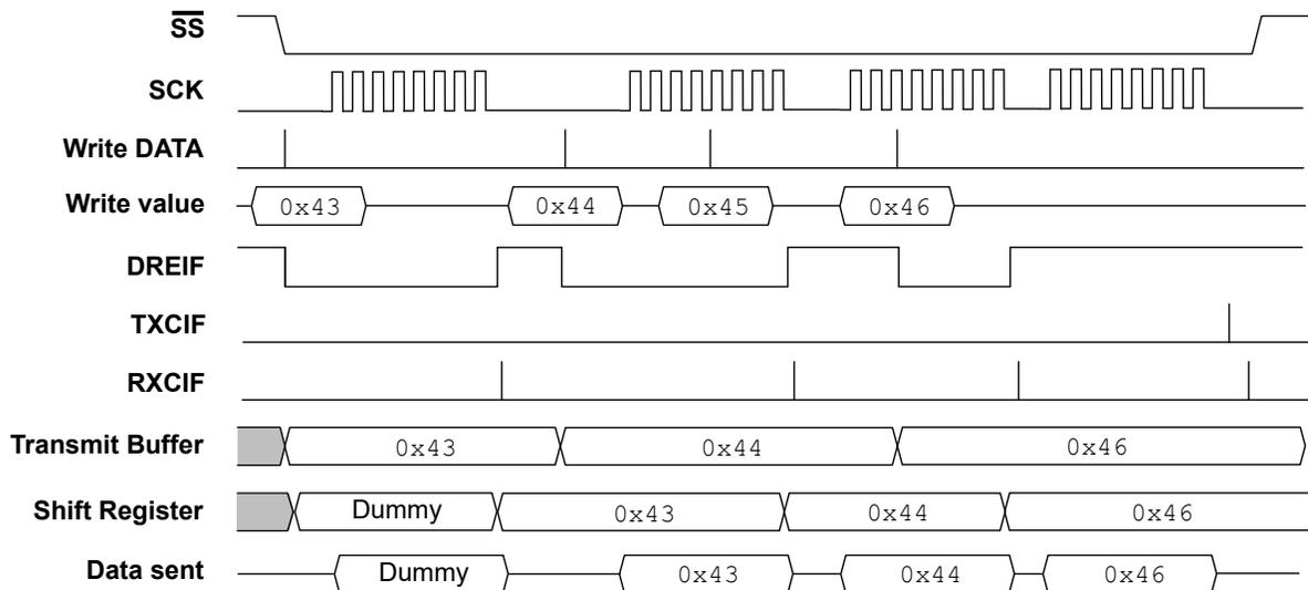
When the Wait for Receive (BUFWR) bit in SPIn.CTRLB is written to '0', all writes to the Data (SPIn.DATA) register go to the Transmit Data Buffer register. The figure above shows that the value 0x43 is written to the Data (SPIn.DATA) register but not immediately transferred to the shift register,
