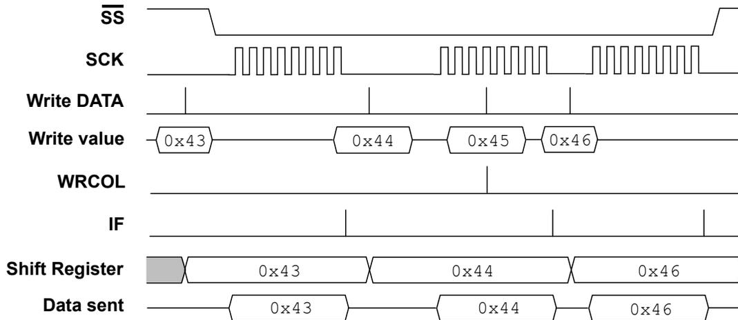
The figure above shows three transfers and one write to the DATA register while the SPI is busy with a transfer. This write will be ignored, and the Write Collision (WRCOL) flag in SPIn.INTFLAGS is set.
