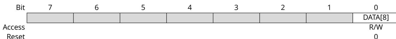
**Bit 0 – DATA[8]** Transmit Data Register High Byte
