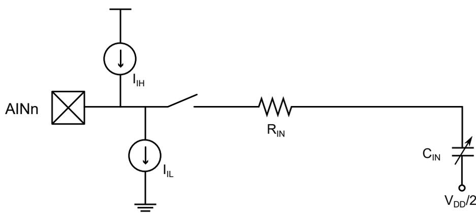
If a source with high impedance is used, the sampling time may need to be increased. The required sample time will depend on how long the source needs to charge the  $C_{IN}$  capacitor and can be configured using the Sample Duration (SAMPDUR) bit field in the Control E (ADCn.CTRLE) register.
