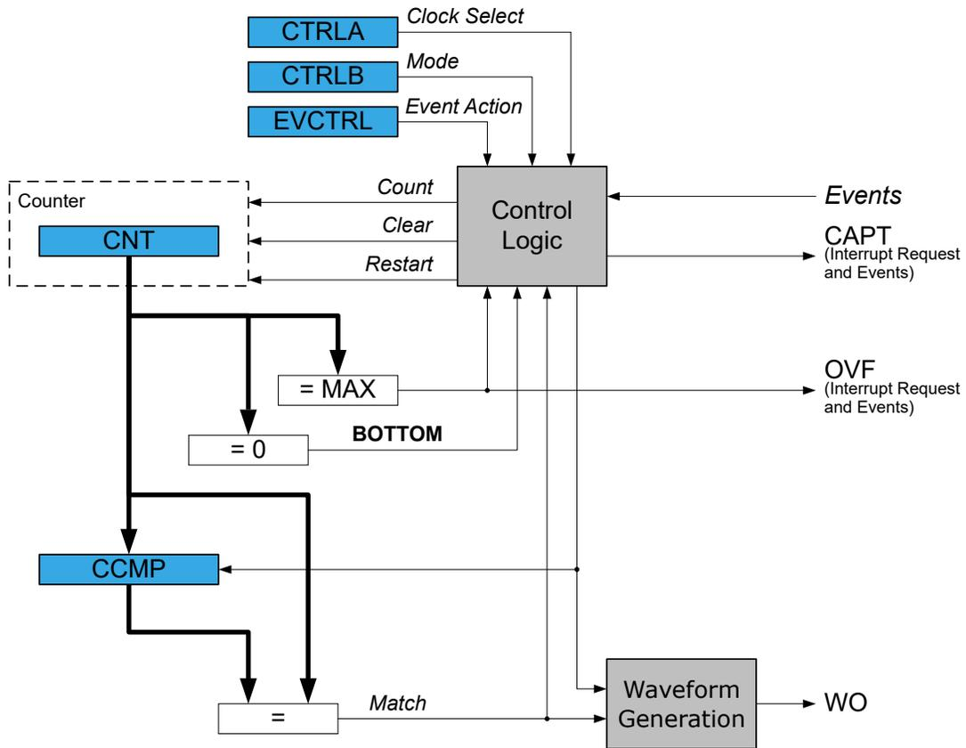
The timer/counter can be clocked from the Peripheral Clock (CLK\_PER), from a 16-bit Timer/Counter type A (CLK\_TCA) or the Event System (EVSYS).
