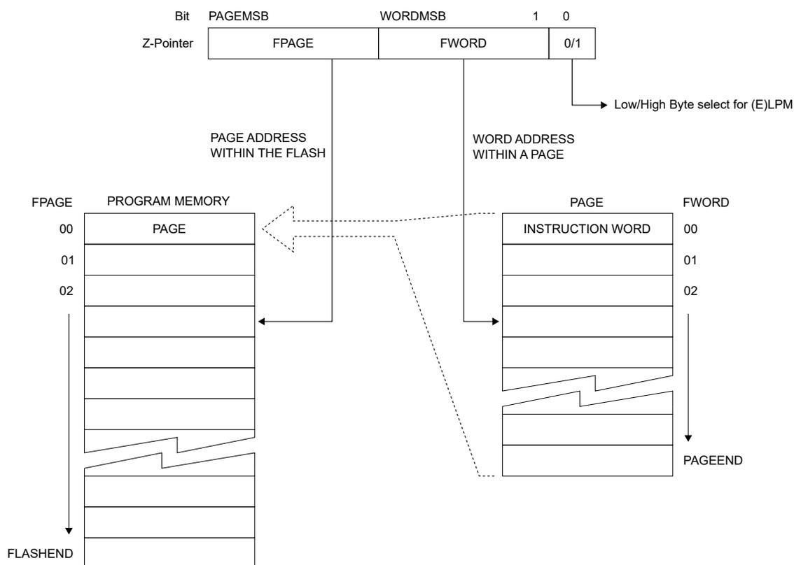
The Flash is word-accessed and organized in pages, so the Address Pointer can be treated as having two sections, as shown in the figure above. The word address in the page (**FWORD**) is held by the Least Significant bits (LSb) in the Address Pointer, while the Most Significant bits (MSb) in the Address Pointer hold the Flash page address (**FPAGE**). **FWORD** and **FPAGE** hold an absolute address to a word in the Flash.
