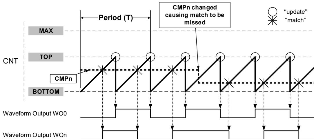
The figure below shows how changing  $CMPn$  during run-time can invert the waveform.
