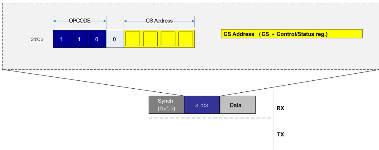
Figure 33-14 shows the data frame transmitted after the SYNCH character and the instruction frames. The STCS instruction byte can immediately be followed by the data byte. There is no response generated from the STCS instruction, as is the case for the ST and STS instructions.
