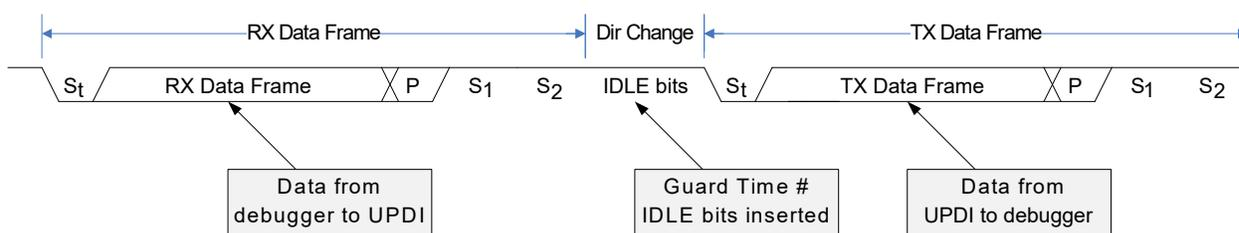
The UPDI guard time is the minimum Idle time that the connected debugger will experience when waiting for data from the UPDI. The maximum Idle time is the same as time-out. When the synchronization time plus the data bus accessing time is longer than the guard time, the Idle time before a transmission will be more than the expected guard time.
