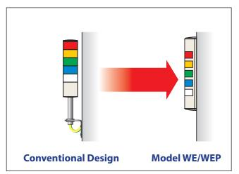
Patlite has perfected a 37.5mm-thin design that significantly enhances integration with the equipment as a built-in signal system.
