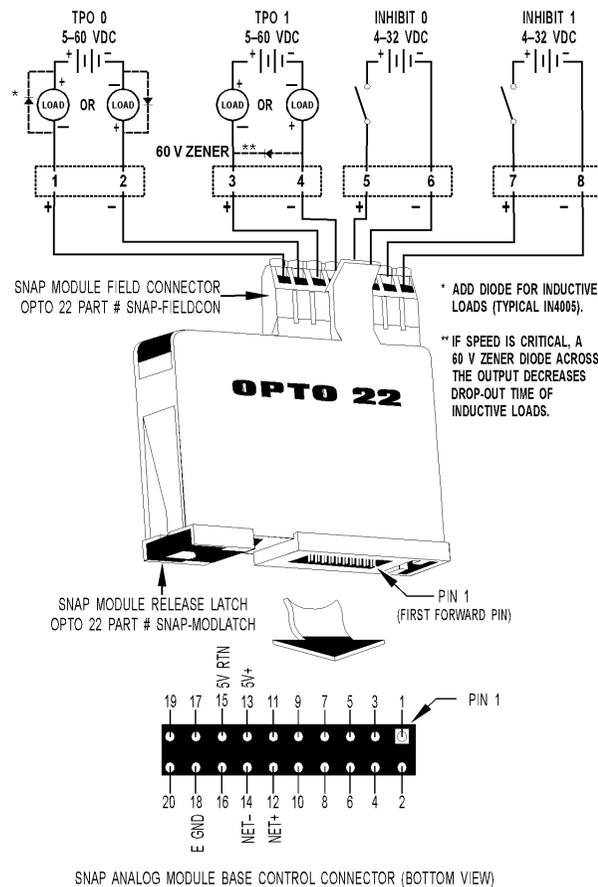
IMPORTANT: The mounting rack connector has 24 pins; the module connector has 20 pins. The extra pins on the mounting rack connector prevent misalignment of the module during installation.
