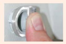
1. Position the disassembly tool over the latch and push to unlock.
