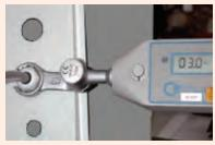
5. Re-tighten the cap nut with prescribed torque.
