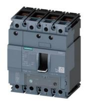
circuit breaker 3VA1 IEC frame 160 breaking capacity class S Icu=36kA @ 415V 4-pole, line protection TM240, ATAM, In=40A overload protection Ir=28A...40A short-circuit protection Ii=5...10 x In N conductor unprotected nut keeper kit
