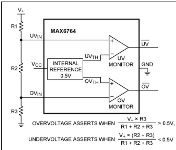
Figure 5. Window detector circuit.
