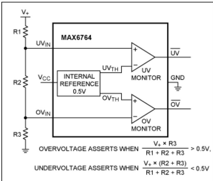
Figure 5. Window detector circuit.
