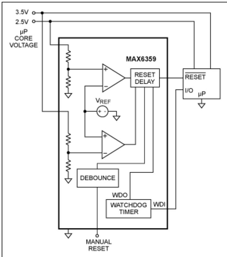
Figure 9. Multiple-supply reset monitoring.
