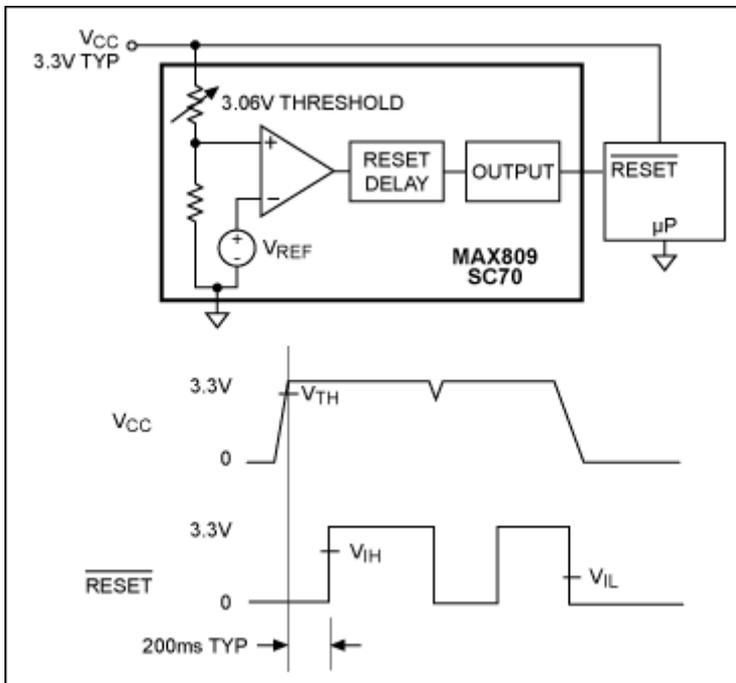
Figure 3. Integrated reset circuit.
