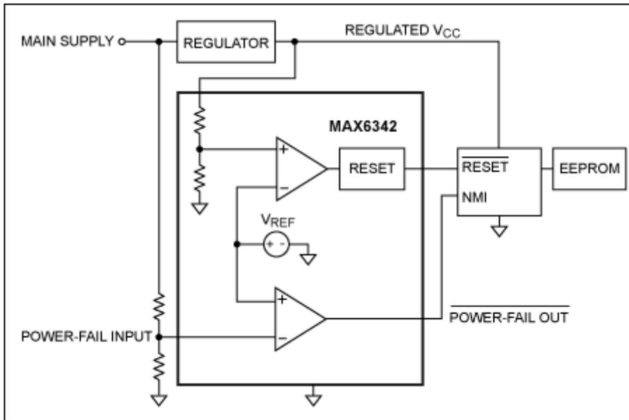
Figure 6. Power-fail/low-battery indicator.
