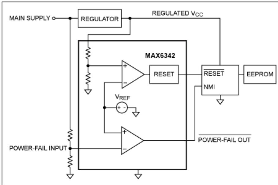
Figure 6. Power-fail/low-battery indicator.
