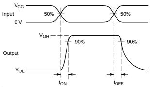
Figure 5.  $t_{ON}/t_{OFF}$
