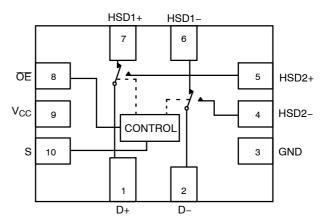
Figure 2. Pin Connections and Logic Diagram (NLAS7222C, Top View)
