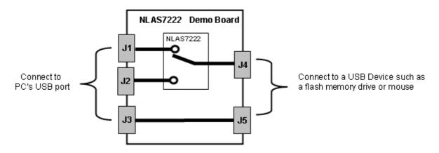
Figure 9. Block Diagram of the NLAS7222B USB Demo Board
