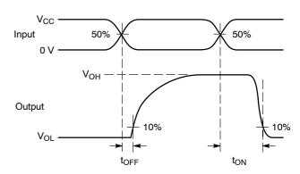
Figure 6. t<sub>ON</sub>/t<sub>OFF</sub>
