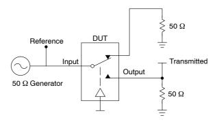
Channel switch control/s test socket is normalized. Off isolation is measured across an off channel. On loss is the bandwidth of an On switch.  $V_{\rm ISO}$ , Bandwidth and  $V_{\rm ONL}$  are independent of the input signal direction.
