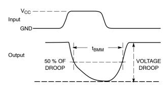
Figure 4. t<sub>BBM</sub> (Time Break-Before-Make)
