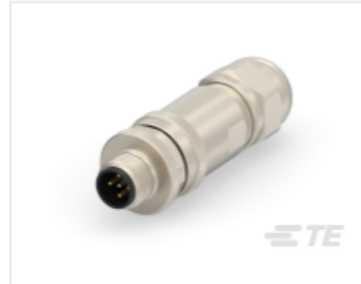
TE Part #T4111011051-000 M12 M, 5P GOLD A_CODE S SHIELDED PG7
