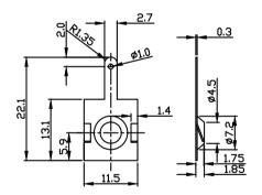
Marked tolerances: according to drawing specifications. Other tolerance: +/- 0.2mm.
