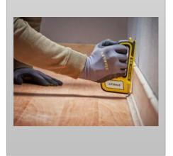
COMPATIBLE FASTENINGS: Fires STANLEY® Type-A staples in 6mm - 10mm and Type-J Headed Brad Pins in 10mm.
