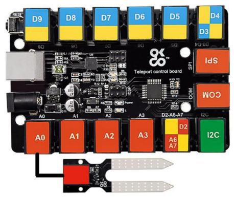
This module is compatible with the TS2178 TelePort control board.
