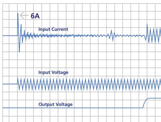
Figure 3: Input inrush current
