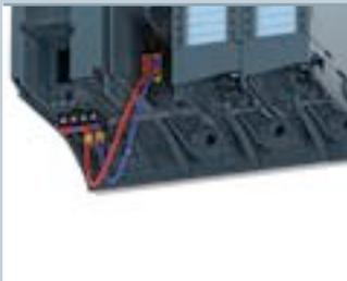
Insert the plug into the load current supply, and wire the load current supply with the CPU.
