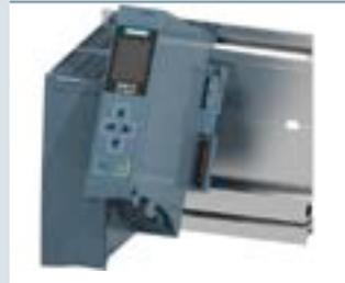
Hook the CPU onto the mounting rail and screw tight.
