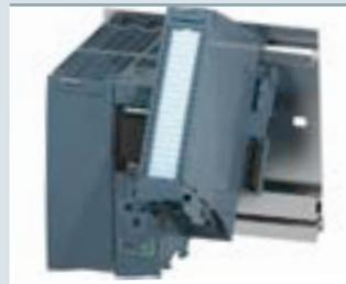
Attach the digital input module to the mounting rail. Ensure the rear of the module is plugged into the U-connector. Screw the module tight.
