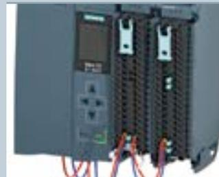
Insert the four potential bridges between the terminals, and connect terminals 30 and 40, as well as 29 and 39 with each other.
