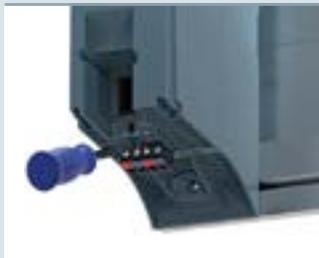
Remove the 4-pin connection plug beneath the load current supply and screw the load current supply tight.
