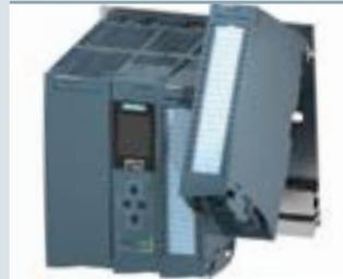
Attach the digital output module to the mounting rail. Ensure the rear of the module is plugged into the U-connector. Screw the module tight.
