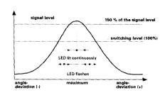
The correct adjustment for maximum receiving signal is achieved by mounting the sensor between the two positions at which the LED starts to flash and adjusting the alignment.
