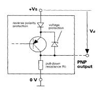
A PNP output acts as an electronic switch from +Vs to the output. The load is switched to 0 Volt. If the output is switched (if "light" is received in a light operate mode or "no light" in a dark operate mode) a current flows from +Vs via the reverse polarity protection diode and the output transistor, through the load to 0 Volt. The voltage between +Vs and the output is called the voltage drop. The voltage protection prevents damage to the output if spikes occur.
