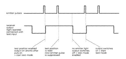
By implementing this, the complete function of the sensor, emitter, receiver and output can be completely monitored. A system failure or an open light path has the same effect on the output state. The proper functioning of a system with a closed light beam, generates an alternating output signal with a defined pulse-pause length as shown in the diagram. Sufficient received sig-
