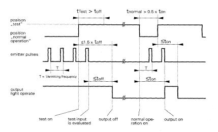
The output is switched off a maximum 1.5 x Toff after the test input is activated. After de-activating the output switches on after a maximum period Ton.
