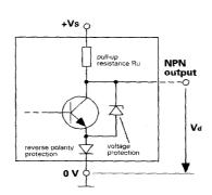
An NPN output acts as an electronic switch from the output to 0 Volt. The load is switched to +Vs. If the output is switched (if "light" is received in a light operate mode or "no light" in a dark operate mode) a current flows from +Vs through the load and via the output transistor and the reverse polarity protection diode to 0 Volt. The voltage between the output and 0 Volt is called the voltage drop. The voltage protection prevents damage to the output if spikes occur.
