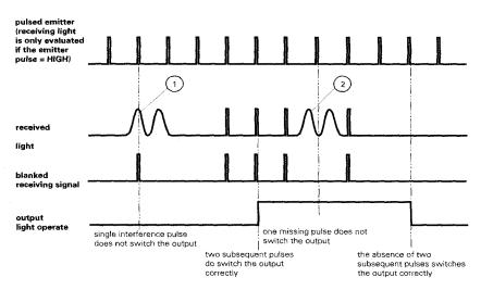
first interference pulse generates a failure, while the emitter pulse is high; the second pulse is blanked
