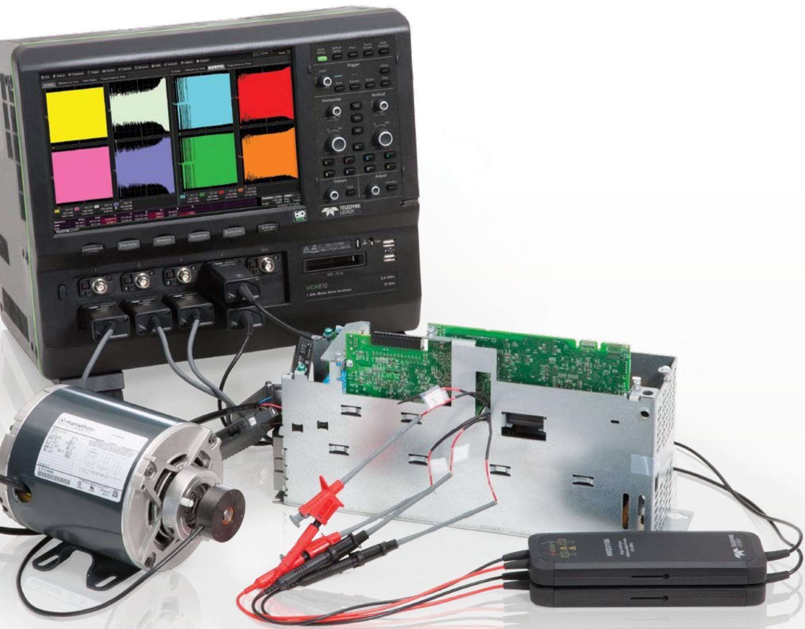
**Differential active probes are like two probes in one. Instead of measuring a test point in relation to a ground point (like single-ended active probes), differential probes measure the difference in voltage of a test point in relation to another test point.**
