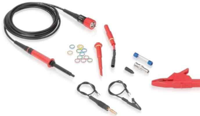
The HVP120 is a high voltage passive probe designed for probing up to 1,000 Vrms and capable of handling up to 6,000 V peak transients. Its fast rise time and excellent frequency response make it suitable for a wide variety of high voltage measurement applications. The HVP120 features a spring loaded probe tip and a variety of standard accessories to make probing high voltages safe and easy.
