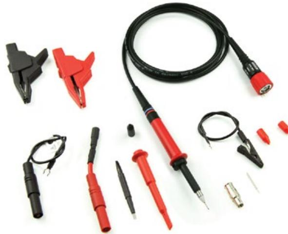
The PPE series includes four fixed-attenuation probes covering a range from 2 kV to 6 kV, and one switchable probe providing  $\div 10/\div 100$  attenuation for voltage inputs up to 1.2 kV. All fixed-attenuation, standard probes automatically rescale compatible Teledyne LeCroy oscilloscopes for the appropriate attenuation of the probe.
