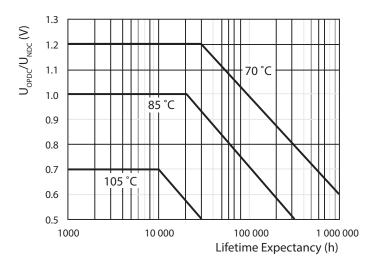
$U_{\tiny NDC}$  is the nominal DC voltage at the nominal temperature of 85 °C, and  $U_{\tiny OPDC}$  is the DC operating voltage in a given application. The ratio between  $U_{\tiny OPDC}$  and  $U_{\tiny NDC}$  will influence the lifespan of the DC-Link capacitor.
