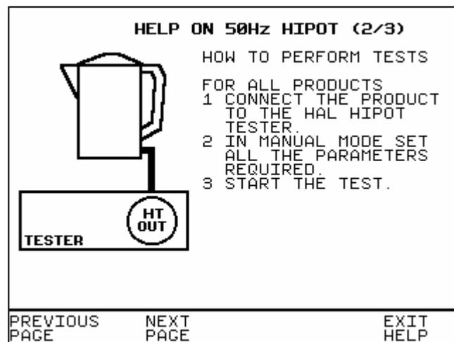
A description of how to connect the test leads and perform the test is provided in a step-by-step format.
