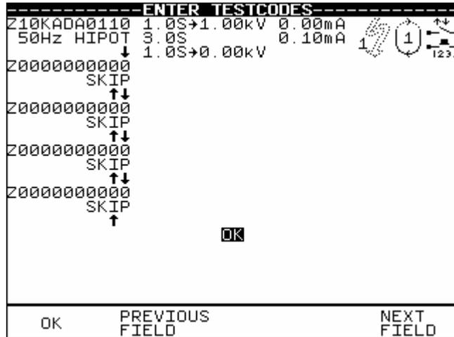
NB: The Test code numbers can also be changed using the encoder. First highlight the test code to be edited, press Green button to bring up the alpha-numeric options on the screen. Use Rotate cursor & Insert keys to enter any combination of test codes sequence. However incorrect test codes will be rejected and activate a warning. See Test code tables for details.
