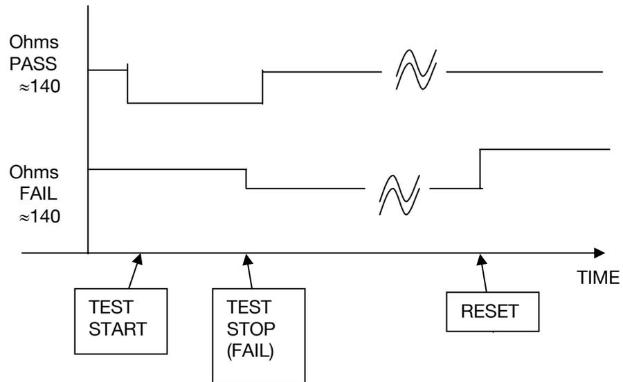
The '**Mode Contacts**' socket may be connected to a remote push-button switch or **no-volt** contact for resetting any fault status on the Hal, by activating the button or contact once only. Any further activation in this mode will default the Hal to its main menu. This is the same for the GREEN button which can be operated externally, in this way.
