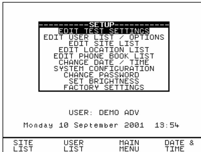
From this menu you can change the way the Tester will operate and also change user levels and sites. Use the encoder to highlight a function and press Green to select the desired option.
