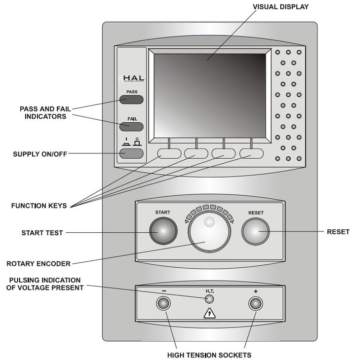
The user is provided with a 320 x 240 1/4 VGA Graphical Liquid Crystal Display (LCD). To the bottom of the screen are four function keys which allow the user fast access to options displayed on the Display
