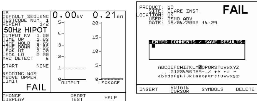
Fail Comments – Use encoder & Insert key to enter in any comments. To skip line or move to next line, highlight Rotate Cursor and turn encoder. Or use barcodes.
