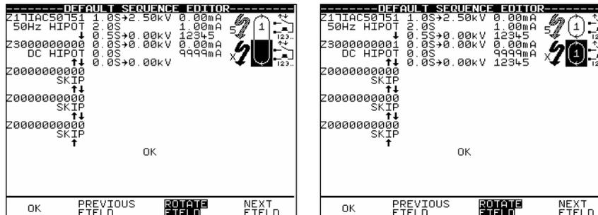
Caution: It must be noted that only the integer(s) selected will conduct the test voltage(s), a blank ' - ' will be by-passed.
