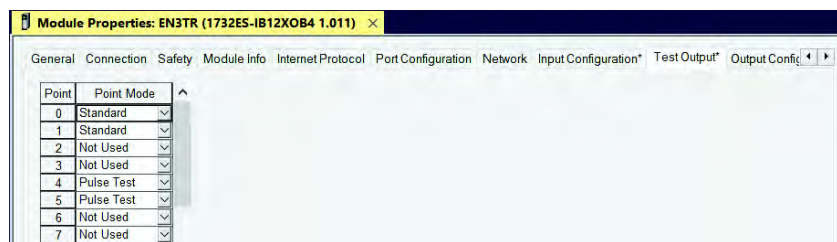
Figure 27 - Module Properties – Test Output
