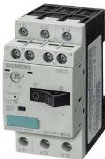
CIRCUIT-BREAKER, SIZE S00, FOR MOTOR PROTECTION, CLASS 10, A REL.2.2...3.2A, N REL.42A, 1NO + 1NC TRANSVERSE, SCREW CONN., STANDARD BREAKING CAPAC.
