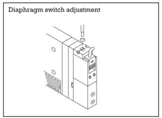
There is a slotted adjuster on top of the vacuum switch for setting actuation vacuum pressure levels.
