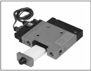
An all in one vacuum generator, silencer, suction filter incorporating an on/off air supply valve. This valve switches the air supply and therefore vacuum on or off via the in-built solenoid. Additionally the unit has a vacuum release (blow-off) valve. This valve switches a positive pressure to quickly release the object being picked. An integral flow control valve provides adjustment to the rate of flow of air used to release the object.
