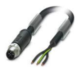
Power cable, 3-position, PVC, black, Plug straight M12 SPEEDCON, S-coded, on free cable end, Cable length: 2 m, For AC current up to 16 A/230 V
