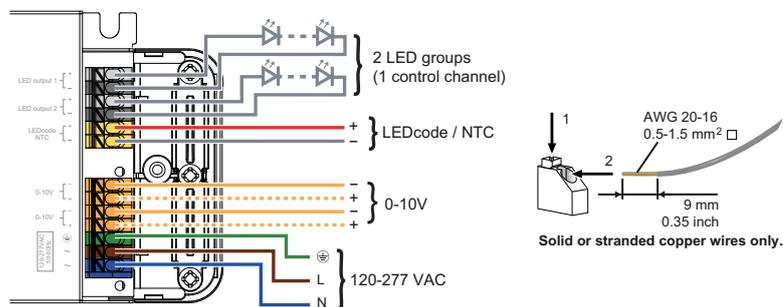
In Europe, use a H03V 0.75mm<sup>2</sup> power cable for 561/A and apply following strip lengths:
