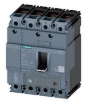
circuit breaker 3VA1 IEC frame 160 breaking capacity class N Icu=25kA @ 415V 4-pole, line protection TM240, ATAM, In=20A overload protection Ir=14A...20A short-circuit protection Ii=8...16 x In N conductor unprotected nut keeper kit
