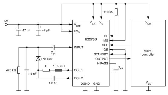
Figure 4-1. Application Circuit 1
