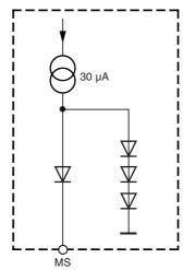
Figure 3-10. Equivalent Circuit of Pin CFE
