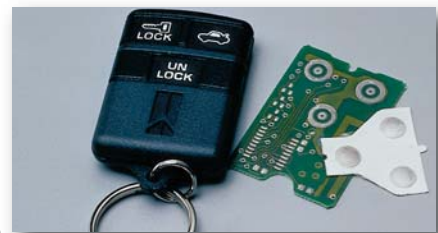
With resistance to high temperatures and humidity, 3M single coated spacer materials effectively maintain registration of metal and polyester domes.
