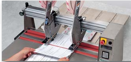
241 A variety of automatic and semi-automatic equipment is available for higher volume applications. For example, apply tape to business forms, literature, bounce back and business reply cards.
