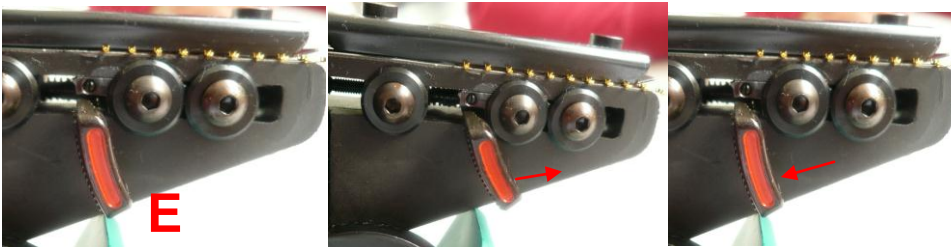
Push in until the locking lever (E) engages with the strip lock and the feed can be effected by yellow feed lever (G, see picture 7). The release lever moves automatically in direction of the arrow during the insertion of the strip of contacts. →
