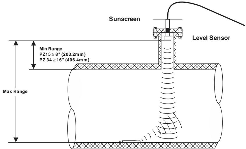
Use a Sensor Sunscreen (option PZS) when sensor is installed indirect sunlight.
