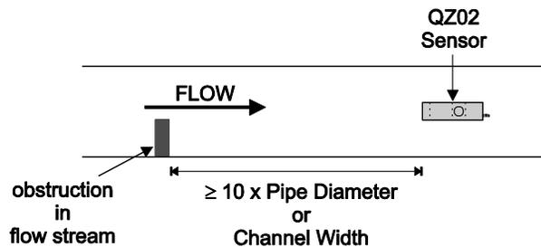
**QZ02L VELOCITY-LEVEL SENSOR MOUNTING**
