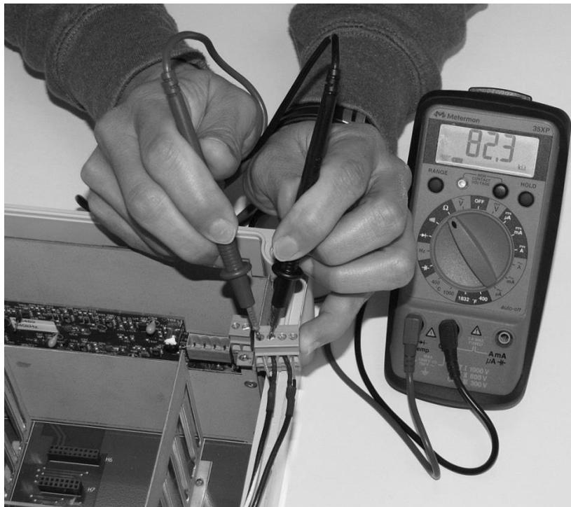
Unplug the 2-pin green sensor terminal from the level board and connect the multimeter to the pins. Resistance should be approximately 10K Ohms for any cable length. High readings indicate an open circuit and low readings indicate a short or partial short.
