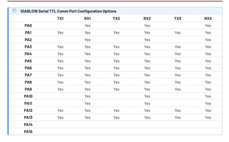
As per the table, not all GPIO can be configured to be every serial port, or RX/TX.
