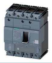
circuit breaker 3VA1 IEC frame 160 breaking capacity class H Icu=70kA @ 415V 4-pole, line protection TM220, ATFM, In=20A overload protection Ir=14A...20A short-circuit protection Ii=16 x In N conductor unprotected clamp connection
