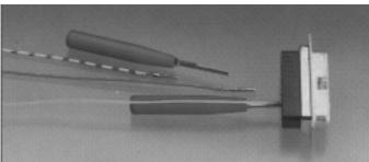
Mounting and dismounting tool for AWG 20-28
