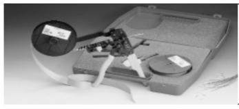
Hand crimping tool for reels with 500 contacts incl. reel holder and adjustable feed AWG 20-28 0.08-0.5 mm<sup>2</sup>
