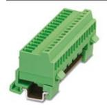
Plug component, Nominal current: 8 A, Rated voltage (III/2): 160 V, Number of positions: 8, Pitch: 3.81 mm, Connection method: Screw connection, Color: green, Contact surface: Tin, Mounting: DIN rail
