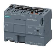
SIMATIC RTU3051C compact low-power RTU; battery or solar-operated; connection external power supply 10.8 V to 28.8 V DC; integrated modem for LTE-M/NB-loTv2; GNSS; connection to TeleControl Server Basic; loadable protocols: DNP3, IEC 60870-5-104, SINAUT ST7 or MQTT; onboard I/Os: 8 DI, 8 DO, 4 AI; FTP client; Ethernet port, configuration/diagnostics via web server, time-of-day synchronization, SMS, email, SD card slot. observe national approvals!
