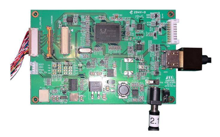
Carefully slide the black part back to lock the FFC into the connector.
